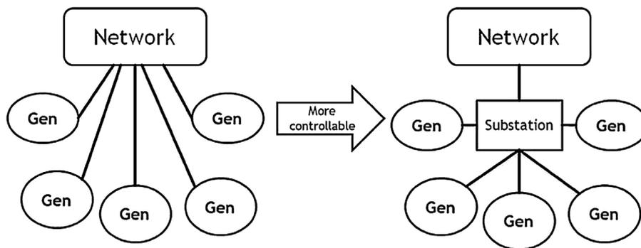
Fig. 6. Traditional (left) method versus the cluster technique (right).
